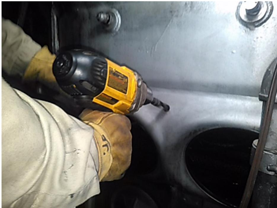
**Figure 2: Drilling Hole in STER Locomotive Air Box**
