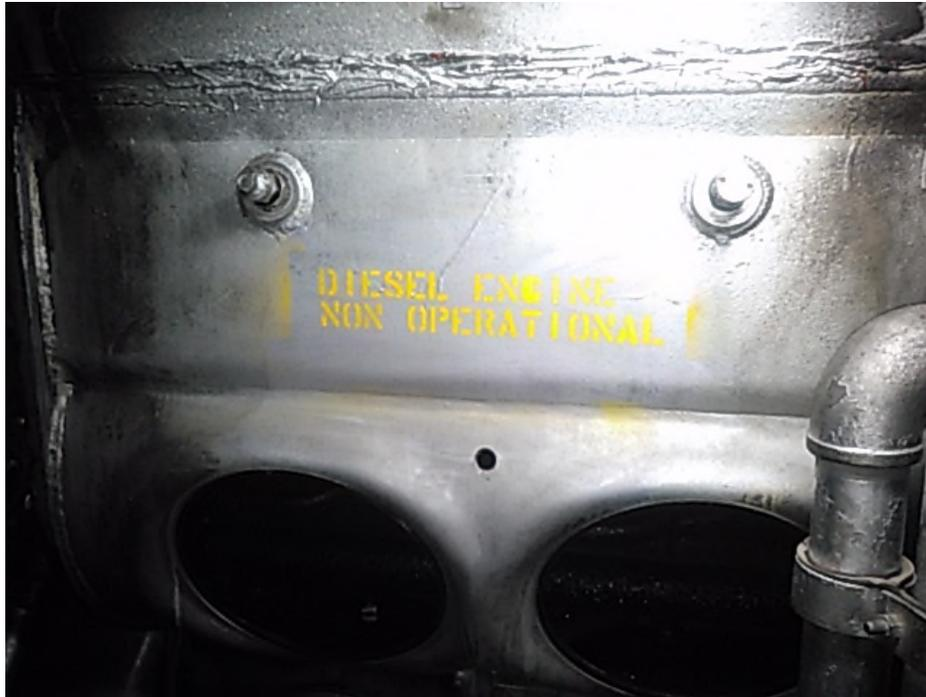
**Figure 3: STER Locomotive Air Box After Hole Drilling**
