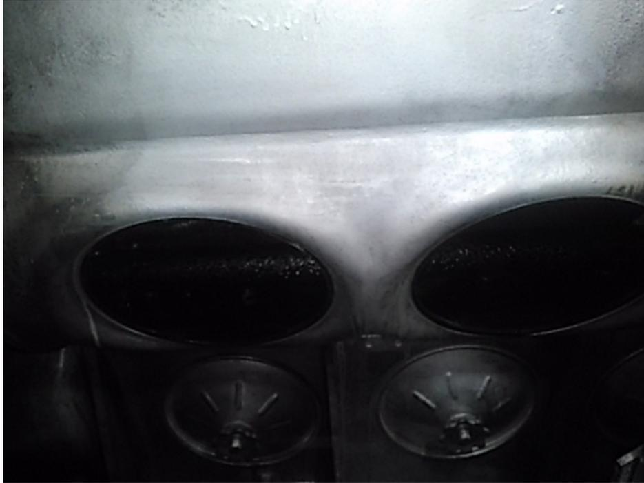
**Figure 1: STER Locomotive Air Box Before Hole Drilling**
