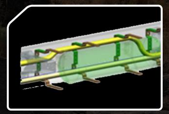
Innovative routing and clipping to keep wiring and air lines separated for reduced damage and faster diagnosis.
