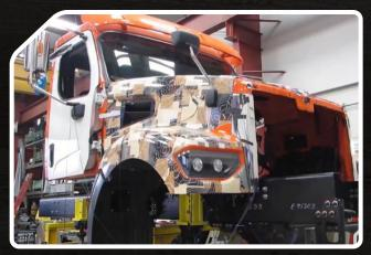
Tested like no other truck before: 400h in the shaker lab representing 800,000 vocational miles; 230,000 door slams representing the lifetime of the truck; multiple cab crush and impact tests.
