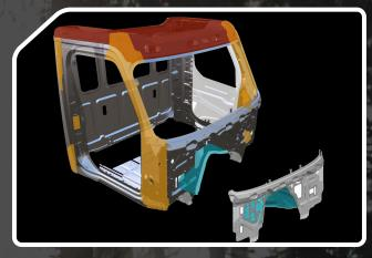
Steel-reinforced aluminum cab designed using advanced topology optimization ensures toughness and durability, while reducing weight.
