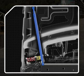
Patented ISO Tech Hood Suspension System isolates the hood from the chassis, absorbing impact from rough terrain on the job site to reduce fatigue on drivers.
