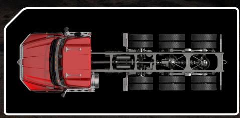
Best-in-class single channel rail strength with RBM rating of 3.7 million inch-lbs. for greater strength, durability and weight savings.
