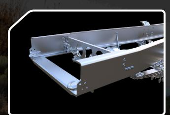
Multiple parent rail front frame extensions for applications requiring front-mounted equipment, such as a snow plow.
