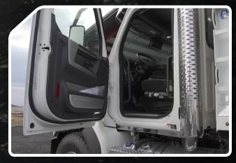
Designed for ergonomic ingress and egress, 70 degree door opening, five hand holds, and optimized staircase step design.
